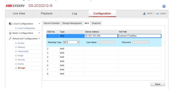
7. Go back to Storage Management, tick the checkbox of the HDD No. and click Format. After it is formatted, the NAS can be used for recording.
