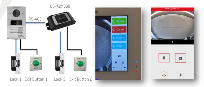
Set the DS-K2M060 secure door control module DIP switch 1 from 0 to 1 and change the door station RS-485 settings according to the below parameters:
